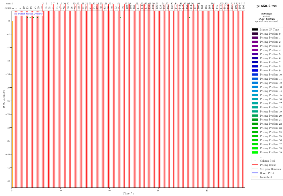
Figure 54: This Plot shows how many variables were generated in a certain pricing round in which time for all nodes of the Branch and Bound tree. The node numbers are shown above the plot and the rounds are in the line below that. Each bar represents the iteration of one pricing problem. Note that the numbers of the pricing problems can have gaps in between, since they could have been aggregated prior to the pricing. Whether those variables are useful is shown by all bars that are below zero, as they mean that the variables of that pricing iteration are in the optimal solution of the Root LP (Root LP Sol) or IP (Incumbent). Finally, the dots show how many columns are taken from the column pool.
