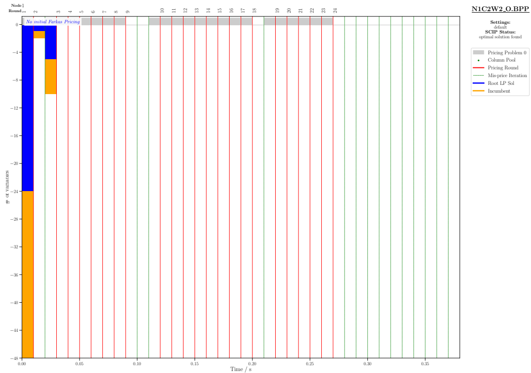
Figure 24: This Plot shows how many variables were generated in a certain pricing round in which time for all nodes of the Branch and Bound tree. The node numbers are shown above the plot and the rounds are in the line below that. Each bar represents the iteration of one pricing problem. Note that the numbers of the pricing problems can have gaps in between, since they could have been aggregated prior to the pricing. Whether those variables are useful is shown by all bars that are below zero, as they mean that the variables of that pricing iteration are in the optimal solution of the Root LP (Root LP Sol) or IP (Incumbent). Finally, the dots show how many columns are taken from the column pool.
